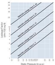
(Based on SMACNA HVAC Air Duct Leakage Test Manual, 1985 Edition, Figure 4-1 'Duct Leakage Classification')
